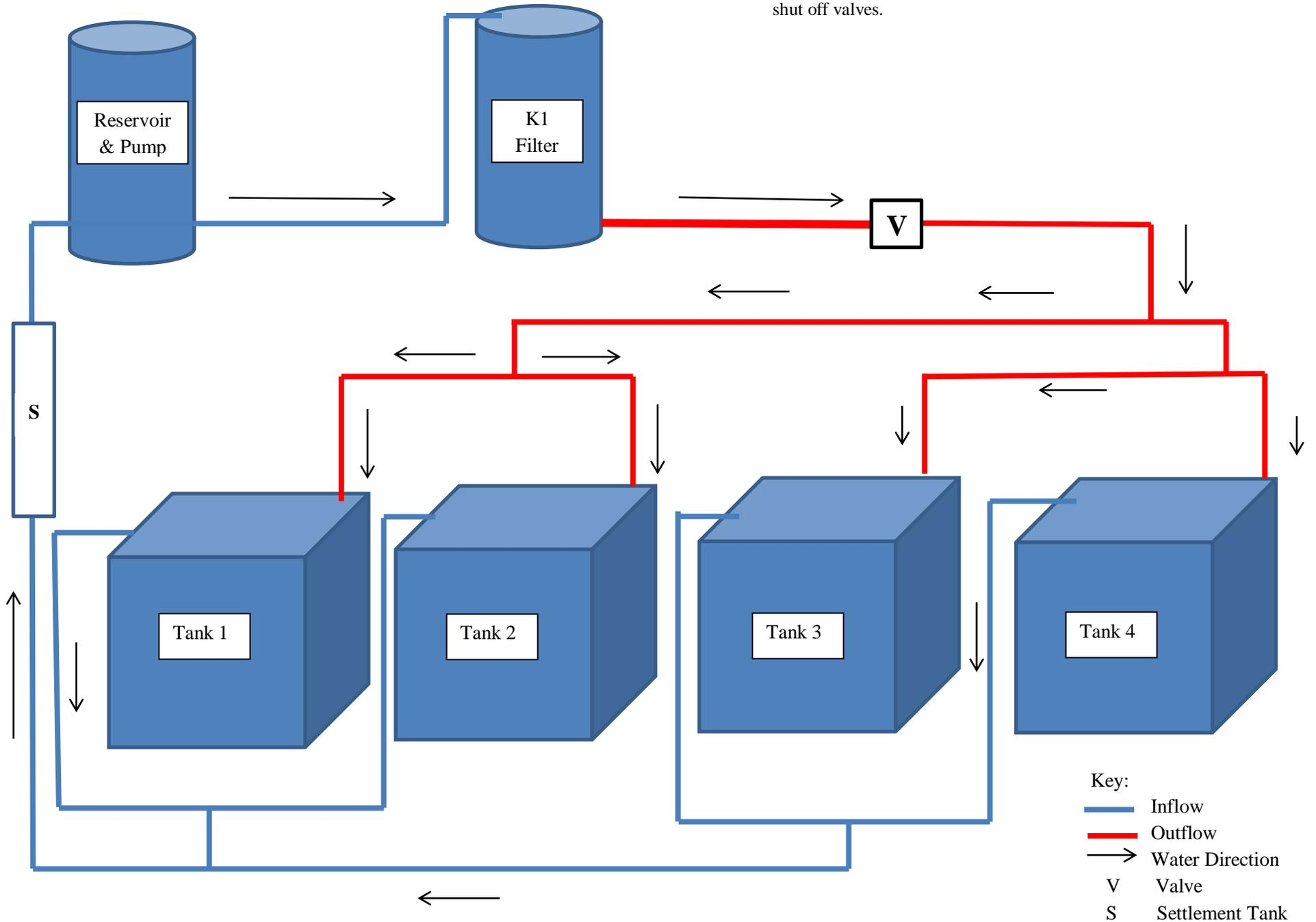
Figure 6. Sump Tanks Filtration Schematic
